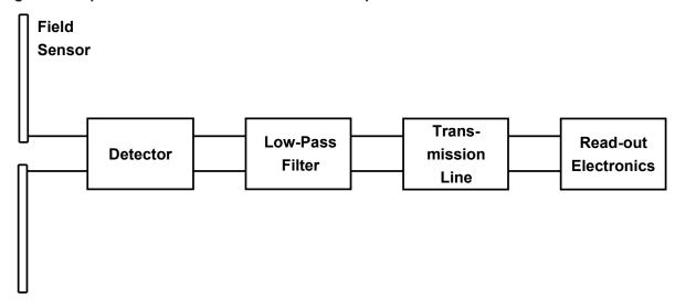
Fig. 1.14 Simplified schematic of a broadband-field probe
