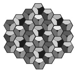
Each cell is hexagonal, with a base station at its centre and configured to provide signals over three sectors of 120 degrees. The shading show how coverage is provided everywhere by use of 12 frequency channels, none of which are used in the adjacent cells.
