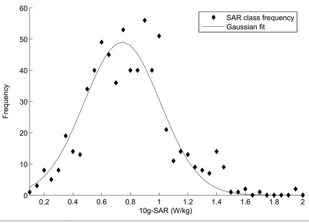
Fig. 1.18 Statistical distribution of maximum psSAR-10 g measured for 668 mobile phones, according to standard EN50361 (CENELEC, 2001)
