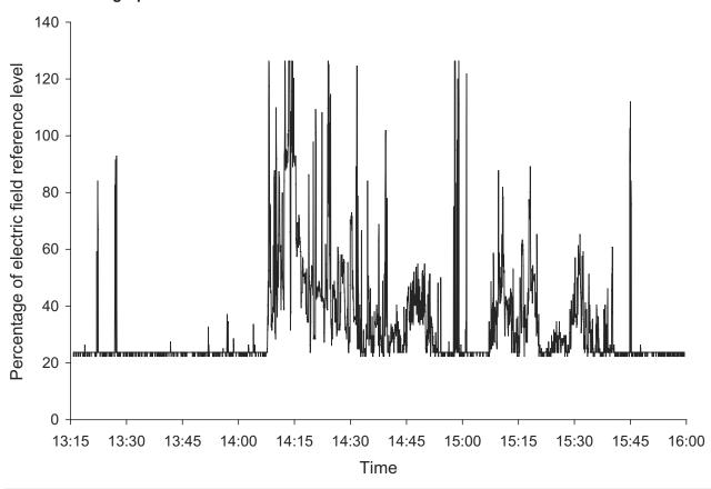
Fig. 1.8 Relative electric-field strength recorded for an engineer operating on a mast supporting antennae for high-power VHF/UHF broadcast transmissions
